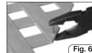
INSERT PINS INTO TRIMMED LATTICE PANEL
