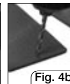
DRILL 3MM HOLE 5MM FROM EDGE
